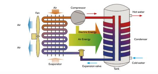
To understand the concept of heat pumps, imagine a refrigerator working in reverse. While a refrigerator removes heat from an enclosed box and expels that heat to the surrounding air, a HPWH takes the heat from surrounding air and transfers it to water in an enclosed tank.
