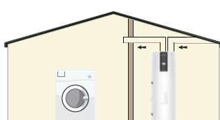
Installation with 2 ducts to the outside
