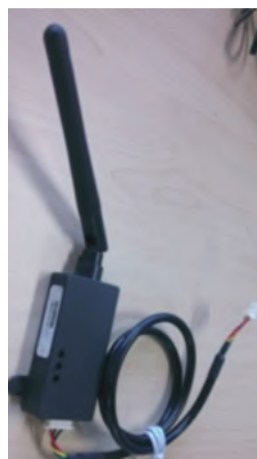
Radio adapter for the indoor unit to be connected to the respective electronic board.
