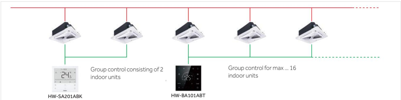
Example of a Wi-Fi module connection, for independent operation of each indoor unit
