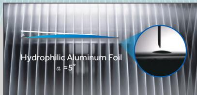
Low-angle hydrophilic aluminium foil speeds up water drainage by 20%.
