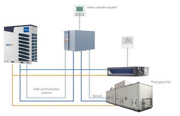
$\label{liquid} Liquid/Gas\ refrigerant\ pipes, only\ the\ liquid\ pipe\ enters\ the\ valve\ box\ and\ then\ continues\ to\ the\ direct\ expansion\ coil.$  The Gas\ pipe\ goes\ directly\ from\ the\ outdoor\ unit\ to\ the\ coil\ inside\ the\ AHU.
