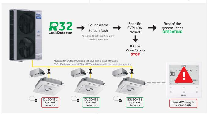
For detailed calculations on Shut-off valve applications and other safety measures compliant with IEC 60335-2-40 regulation, refer to the MRV Selection software.
