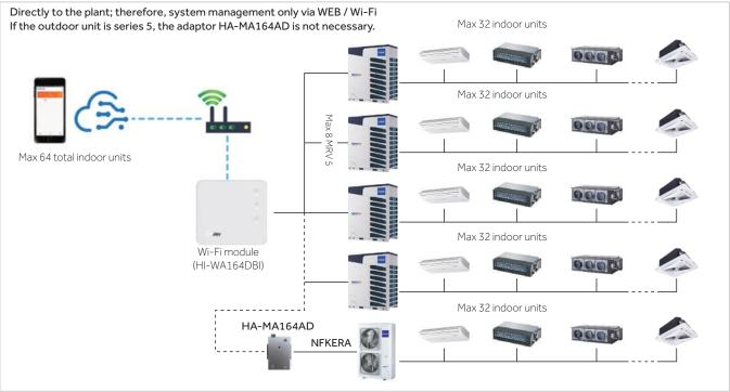
If used independently (not connected to a centrallized controller) it is necessary to provide 12 DC electric supply (not provided by Haier)
