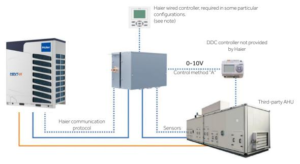
Liquid/Gas refrigerant pipes, only the liquid pipe enters the valve box and then continues to the direct expansion coil. The Gas pipe goes directly from the outdoor unit to the coil inside the AHU.
