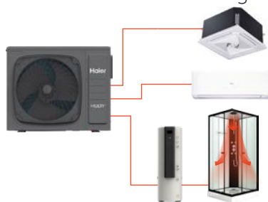
Scenario 2: Domestic Hot Water + AC Heating
