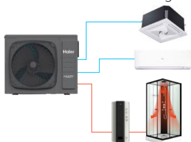
Scenario 5: Domestic Hot Water + AC Cooling
