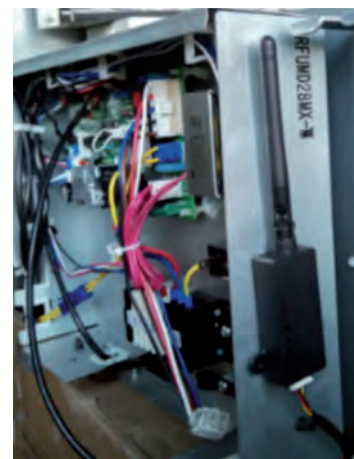
Radio adapter for the indoor unit to be connected to the respective electronic board.
